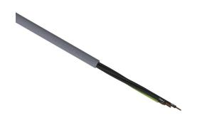
LUTZE Silflex flexible control cable, unshielded, 4 conductors (includes ground), 12 AWG, bare copper, PVC/Nylon conductor insulation material, black with white numbers and green/yellow ground, PVC jacket, gray, cut to length.
