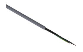
LUTZE Silflex flexible control cable, unshielded, 3 conductors (includes ground), 12 AWG, bare copper, PVC/Nylon conductor insulation material, black with white numbers and green/yellow ground, PVC jacket, gray, cut to length.
