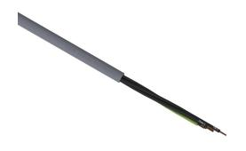
LUTZE Silflex flexible control cable, unshielded, 4 conductors (includes ground), 10 AWG, bare copper, PVC/Nylon conductor insulation material, black with white numbers and green/yellow ground, PVC jacket, gray, cut to length.
