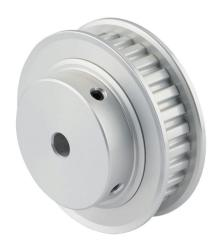
Sung-II Machinery timing pulley, aluminum, 1/5in XL pitch, 30 tooth, 1.91in pitch diameter, 1/4in bore, hub with flanges. For use with 3/8in wide belt.
