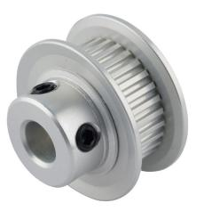
Sung-Il Machinery timing pulley, aluminum, 0.08in MXL pitch, 30 tooth, 0.764in pitch diameter, 1/4in bore, hub with flanges. For use with 1/4in wide belt.
