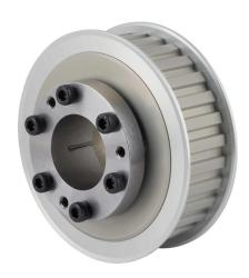
Sung-II Machinery timing pulley, aluminum, 3/8in L pitch, 30 tooth, 3.581in pitch diameter, 1-1/4in bore, no hub with flanges. For use with 1in wide belt. QD bushing included.
