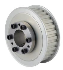
Sung-II Machinery timing pulley, aluminum, 3/8in L pitch, 30 tooth, 3.581in pitch diameter, 1-1/8in bore, no hub with flanges. For use with 1in wide belt. QD bushing included.
