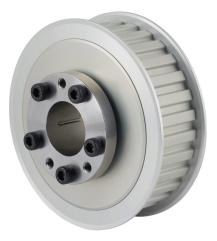
Sung-Il Machinery timing pulley, aluminum, 3/8in L pitch, 30 tooth, 3.581in pitch diameter, 1in bore, no hub with flanges. For use with 1in wide belt. QD bushing included.
