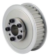
Sung-Il Machinery timing pulley, aluminum, 3/8in L pitch, 30 tooth, 3.581in pitch diameter, 7/8in bore, no hub with flanges. For use with 1in wide belt. QD bushing included.
