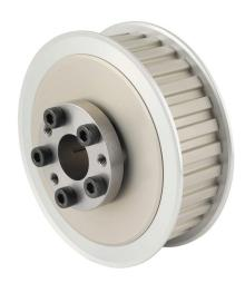
Sung-Il Machinery timing pulley, aluminum, 3/8in L pitch, 30 tooth, 3.581in pitch diameter, 3/4in bore, no hub with flanges. For use with 1in wide belt. QD bushing included.
