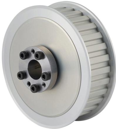
Sung-II Machinery timing pulley, aluminum, 3/8in L pitch, 30 tooth, 3.581in pitch diameter, 5/8in bore, no hub with flanges. For use with 1in wide belt. QD bushing included.
