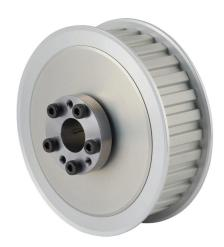
Sung-Il Machinery timing pulley, aluminum, 3/8in L pitch, 30 tooth, 3.581in pitch diameter, 5/8in bore, no hub with flanges. For use with 1in wide belt. QD bushing included.
