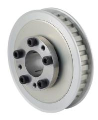
Sung-Il Machinery timing pulley, aluminum, 3/8in L pitch, 30 tooth, 3.581in pitch diameter, 1in bore, no hub with flanges. For use with 1/2in wide belt. QD bushing included.
