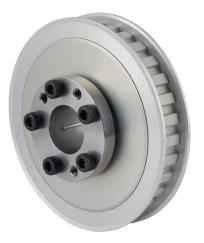
Sung-Il Machinery timing pulley, aluminum, 3/8in L pitch, 30 tooth, 3.581in pitch diameter, 7/8in bore, no hub with flanges. For use with 1/2in wide belt. QD bushing included.
