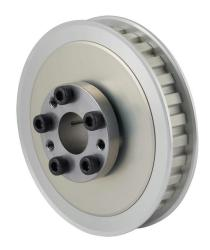
Sung-Il Machinery timing pulley, aluminum, 3/8in L pitch, 30 tooth, 3.581in pitch diameter, 3/4in bore, no hub with flanges. For use with 1/2in wide belt. QD bushing included.
