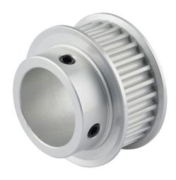
Sung-Il Machinery timing pulley, aluminum, 5mm 5M pitch, 30 tooth, 1.88in pitch diameter, 1-1/8in bore, hub with flanges. For use with 15mm wide belt.
