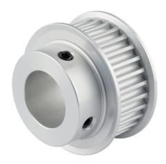
Sung-II Machinery timing pulley, aluminum, 5mm 5M pitch, 30 tooth, 1.88in pitch diameter, 7/8in bore, hub with flanges. For use with 15mm wide belt.
