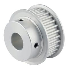
Sung-Il Machinery timing pulley, aluminum, 5mm 5M pitch, 30 tooth, 1.88in pitch diameter, 5/8in bore, hub with flanges. For use with 15mm wide belt.
