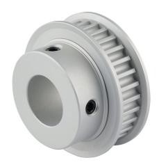
Sung-II Machinery timing pulley, aluminum, 5mm 5M pitch, 30 tooth, 1.88in pitch diameter, 3/4in bore, hub with flanges. For use with 9mm wide belt.
