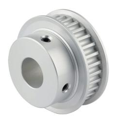
Sung-II Machinery timing pulley, aluminum, 5mm 5M pitch, 30 tooth, 1.88in pitch diameter, 5/8in bore, hub with flanges. For use with 9mm wide belt.
