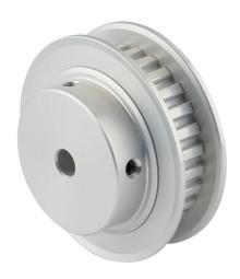
Sung-II Machinery timing pulley, aluminum, 1/5in XL pitch, 28 tooth, 1.783in pitch diameter, 1/4in bore, hub with flanges. For use with 3/8in wide belt.
