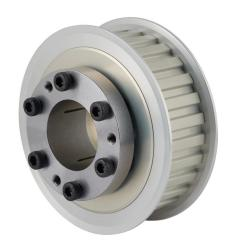
Sung-II Machinery timing pulley, aluminum, 3/8in L pitch, 28 tooth, 3.342in pitch diameter, 1-1/4in bore, no hub with flanges. For use with 1in wide belt. QD bushing included.
