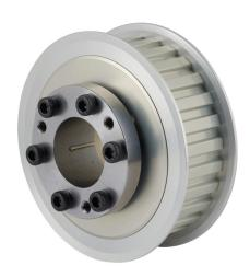
Sung-II Machinery timing pulley, aluminum, 3/8in L pitch, 28 tooth, 3.342in pitch diameter, 1-1/8in bore, no hub with flanges. For use with 1in wide belt. QD bushing included.
