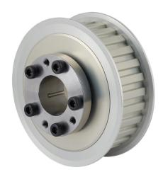
Sung-Il Machinery timing pulley, aluminum, 3/8in L pitch, 28 tooth, 3.342in pitch diameter, 1in bore, no hub with flanges. For use with 1in wide belt. QD bushing included.
