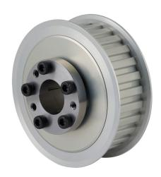
Sung-Il Machinery timing pulley, aluminum, 3/8in L pitch, 28 tooth, 3.342in pitch diameter, 7/8in bore, no hub with flanges. For use with 1in wide belt. QD bushing included.
