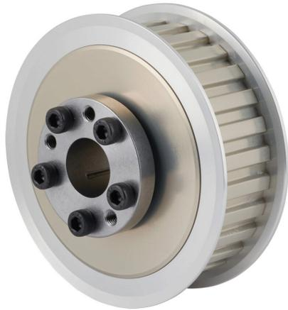
Sung-II Machinery timing pulley, aluminum, 3/8in L pitch, 28 tooth, 3.342in pitch diameter, 3/4in bore, no hub with flanges. For use with 1in wide belt. QD bushing included.
