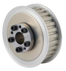
Sung-Il Machinery timing pulley, aluminum, 3/8in L pitch, 28 tooth, 3.342in pitch diameter, 3/4in bore, no hub with flanges. For use with 1in wide belt. QD bushing included.
