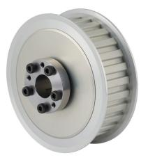
Sung-Il Machinery timing pulley, aluminum, 3/8in L pitch, 28 tooth, 3.342in pitch diameter, 5/8in bore, no hub with flanges. For use with 1in wide belt. QD bushing included.
