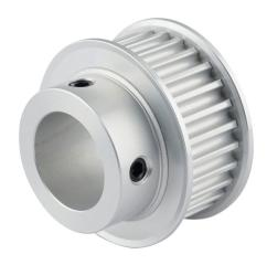
Sung-II Machinery timing pulley, aluminum, 5mm 5M pitch, 28 tooth, 1.754in pitch diameter, 7/8in bore, hub with flanges. For use with 15mm wide belt.
