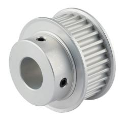
Sung-Il Machinery timing pulley, aluminum, 5mm 5M pitch, 28 tooth, 1.754in pitch diameter, 5/8in bore, hub with flanges. For use with 15mm wide belt.
