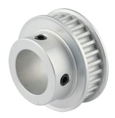
Sung-Il Machinery timing pulley, aluminum, 5mm 5M pitch, 28 tooth, 1.754in pitch diameter, 7/8in bore, hub with flanges. For use with 9mm wide belt.
