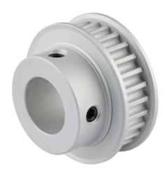
Sung-Il Machinery timing pulley, aluminum, 5mm 5M pitch, 28 tooth, 1.754in pitch diameter, 3/4in bore, hub with flanges. For use with 9mm wide belt.
