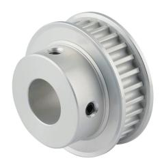
Sung-Il Machinery timing pulley, aluminum, 5mm 5M pitch, 28 tooth, 1.754in pitch diameter, 5/8in bore, hub with flanges. For use with 9mm wide belt.
