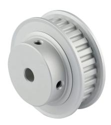
Sung-II Machinery timing pulley, aluminum, 1/5in XL pitch, 26 tooth, 1.655in pitch diameter, 1/4in bore, hub with flanges. For use with 3/8in wide belt.
