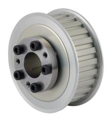
Sung-Il Machinery timing pulley, aluminum, 3/8in L pitch, 26 tooth, 3.104in pitch diameter, 7/8in bore, no hub with flanges. For use with 1in wide belt. QD bushing included.
