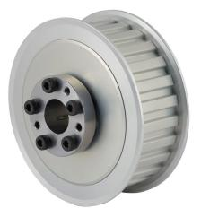
Sung-Il Machinery timing pulley, aluminum, 3/8in L pitch, 26 tooth, 3.104in pitch diameter, 5/8in bore, no hub with flanges. For use with 1in wide belt. QD bushing included.
