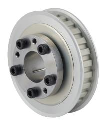
Sung-Il Machinery timing pulley, aluminum, 3/8in L pitch, 26 tooth, 3.104in pitch diameter, 1in bore, no hub with flanges. For use with 1/2in wide belt. QD bushing included.
