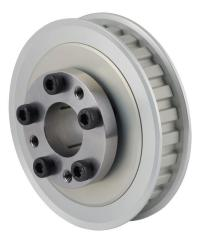
Sung-Il Machinery timing pulley, aluminum, 3/8in L pitch, 26 tooth, 3.104in pitch diameter, 7/8in bore, no hub with flanges. For use with 1/2in wide belt. QD bushing included.
