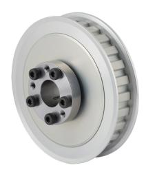
Sung-Il Machinery timing pulley, aluminum, 3/8in L pitch, 26 tooth, 3.104in pitch diameter, 5/8in bore, no hub with flanges. For use with 1/2in wide belt. QD bushing included.
