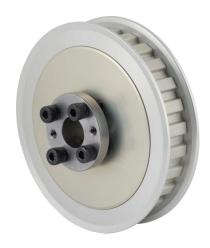
Sung-Il Machinery timing pulley, aluminum, 3/8in L pitch, 26 tooth, 3.104in pitch diameter, 1/2in bore, no hub with flanges. For use with 1/2in wide belt. QD bushing included.
