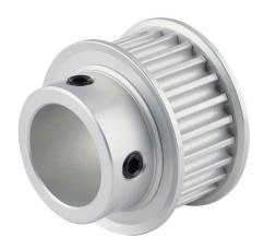
Sung-Il Machinery timing pulley, aluminum, 5mm 5M pitch, 25 tooth, 1.566in pitch diameter, 7/8in bore, hub with flanges. For use with 15mm wide belt.
