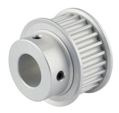
Sung-Il Machinery timing pulley, aluminum, 5mm 5M pitch, 25 tooth, 1.566in pitch diameter, 5/8in bore, hub with flanges. For use with 15mm wide belt.
