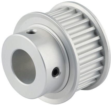
Sung-II Machinery timing pulley, aluminum, 5mm 5M pitch, 25 tooth, 1.566in pitch diameter, 5/8in bore, hub with flanges. For use with 15mm wide belt.
