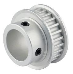
Sung-Il Machinery timing pulley, aluminum, 5mm 5M pitch, 25 tooth, 1.566in pitch diameter, 7/8in bore, hub with flanges. For use with 9mm wide belt.
