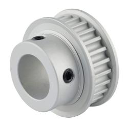
Sung-Il Machinery timing pulley, aluminum, 5mm 5M pitch, 25 tooth, 1.566in pitch diameter, 3/4in bore, hub with flanges. For use with 9mm wide belt.
