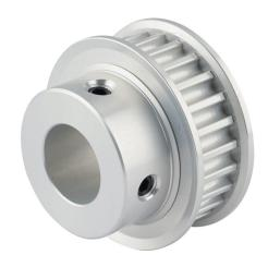
Sung-Il Machinery timing pulley, aluminum, 5mm 5M pitch, 25 tooth, 1.566in pitch diameter, 5/8in bore, hub with flanges. For use with 9mm wide belt.
