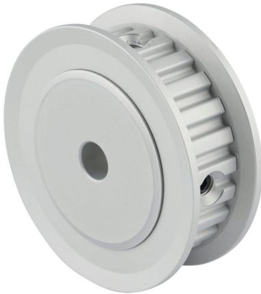
Sung-II Machinery timing pulley, aluminum, 1/5in XL pitch, 24 tooth, 1.528in pitch diameter, 1/4in bore, no hub with flanges. For use with 3/8in wide belt.
