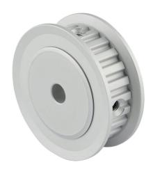
Sung-Il Machinery timing pulley, aluminum, 1/5in XL pitch, 24 tooth, 1.528in pitch diameter, 1/4in bore, no hub with flanges. For use with 3/8in wide belt.
