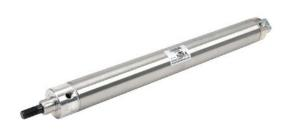
NITRA pneumatic cylinder, non-repairable, 1-1/2in bore, 7/16in rod diameter, 12in stroke, double acting, rear pivot mount.
