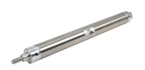
NITRA pneumatic cylinder, non-repairable, 1-1/2in bore, 7/16in rod diameter, 12in stroke, double acting, magnetic piston, rear pivot mount.
