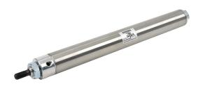
NITRA pneumatic cylinder, non-repairable, 1-1/2in bore, 7/16in rod diameter, 12in stroke, double acting, front nose mount.
