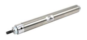
NITRA pneumatic cylinder, non-repairable, 1-1/2in bore, 7/16in rod diameter, 11in stroke, double acting, front nose mount.
