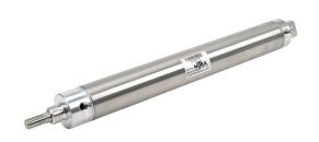
NITRA pneumatic cylinder, non-repairable, 1-1/2in bore, 7/16in rod diameter, 10in stroke, double acting, magnetic piston, rear pivot mount.
