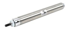
NITRA pneumatic cylinder, non-repairable, 1-1/2in bore, 7/16in rod diameter, 10in stroke, double acting, front nose mount.
